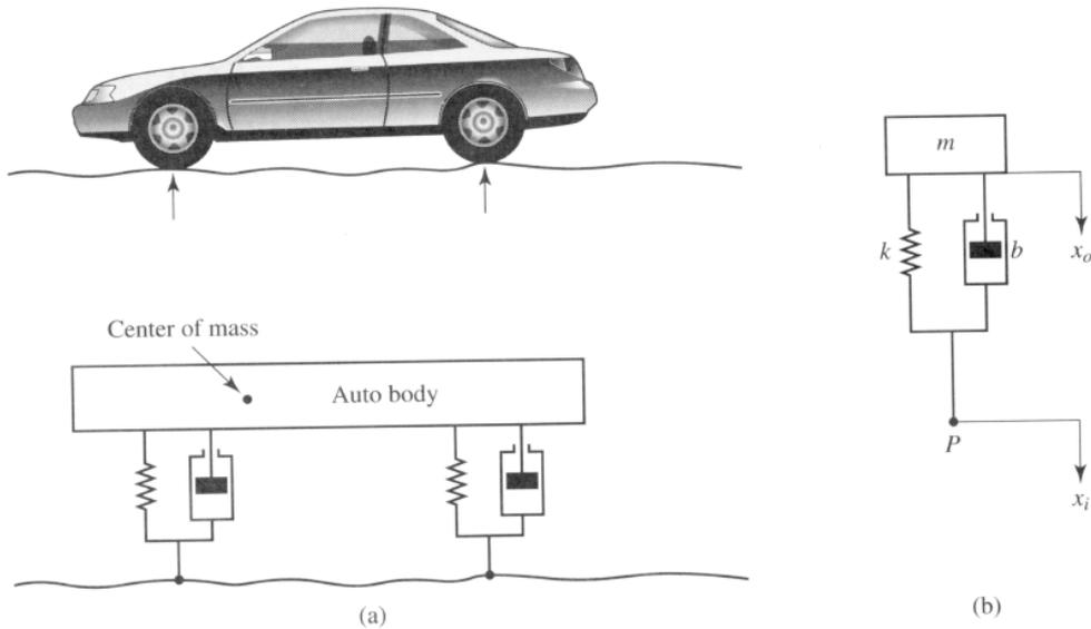
The transfer function of the simplified car suspension system is
