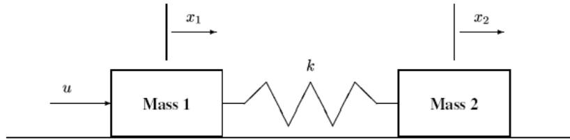
In the system,  $u(t)$  is the input force,  $k = 1$  is the spring constant,  $x_1$  and  $x_2$  are, respectively, the displacements of Mass 1 and Mass 2, which have masses of  $m_1 = m_2 = 1$ . Assume that there is no friction on the surfaces.
