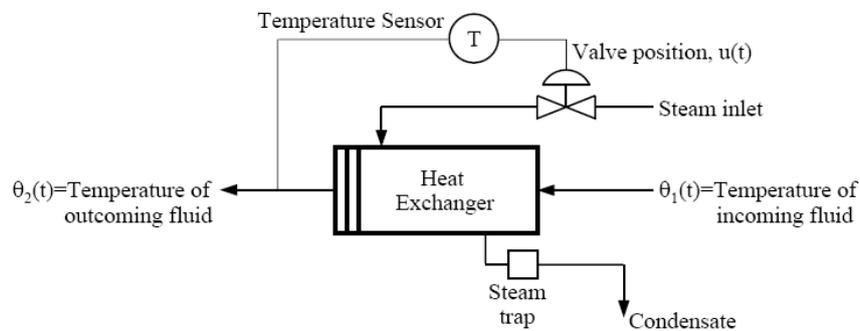
The dynamic behavior of the heat exchanger may be modeled by the following equation:
