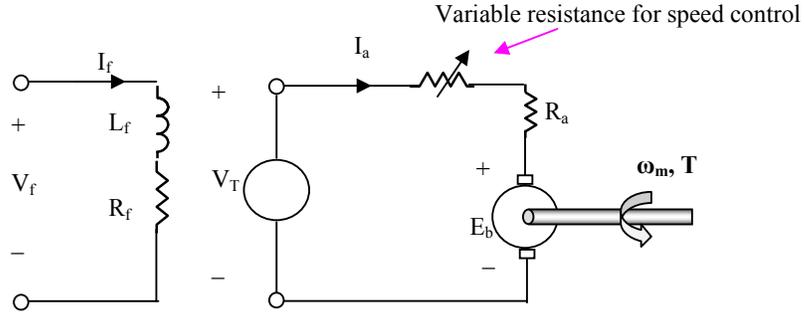
Figure 18: Armature resistance method for speed control
