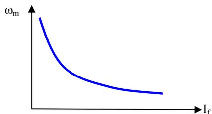
Figure 17: Variation of speed with field current
