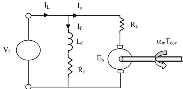
Figure 9: Shunt DC Motor
