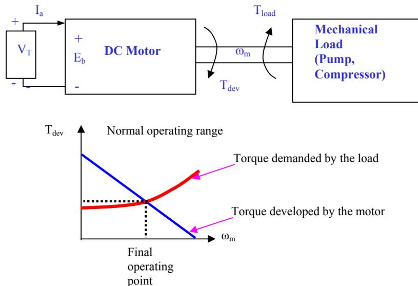
Figure 12: Interaction of the DC Motor and Mechanical Load
