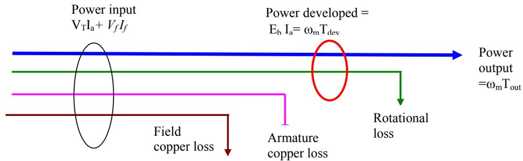
Figure 14: Power flow in a DC motor
