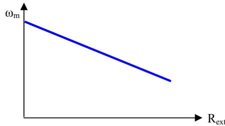
Figure 19: Variation of speed with external armature resistance
