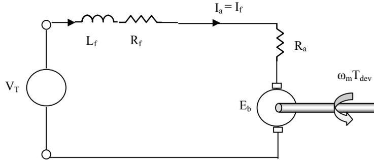
Figure 10 (redrawn): DC Series motor equivalent circuit
