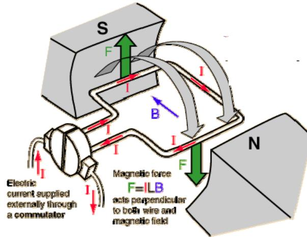
Figure 4: Torque production in a DC motor
