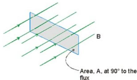
Figure 3: Magnetic flux density
