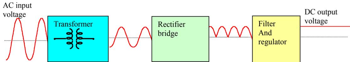
Figure 24: Block diagram of a power supply
