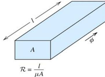
Figure 5: Magnetic circuit
