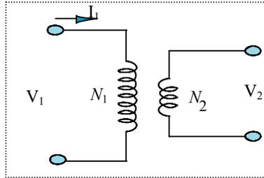
Figure 13(b): Step-down transformer
