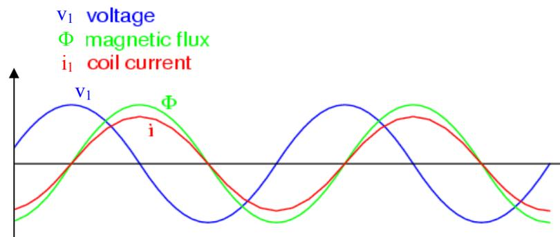
Figure 9: Voltage, current and flux in the primary winding
