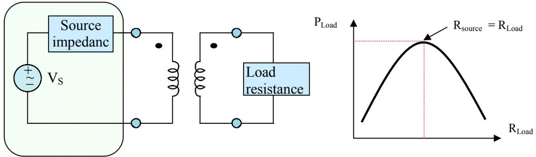
Figure 20: Transformer application for impedance matching
