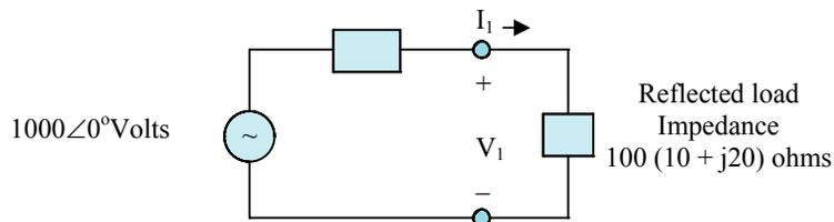
Figure 23: Simplified circuit
