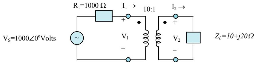
Figure 22: Transformer equivalent circuit for example 4
