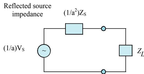
Figure 19: Simplified circuit
