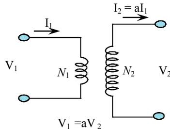
Figure. 12: Ideal transformer equivalent circuit
