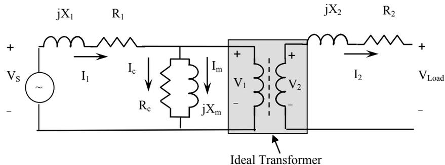
Figure 25: Equivalent circuit of a practical transformer
