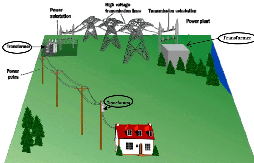
*Figure 8: Transformers in Power Systems*
