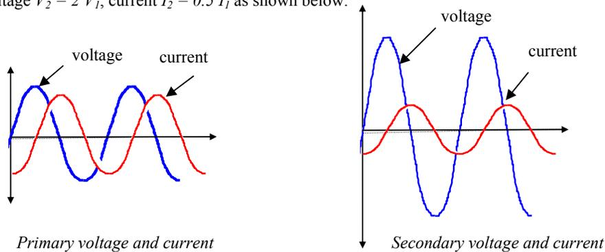
Figure 11: Voltage and current waveforms
