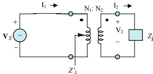
Figure 16: Load impedance as *seen* by the source
