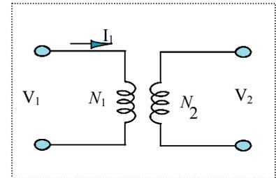
Figure 13(c): Isolation transformer
