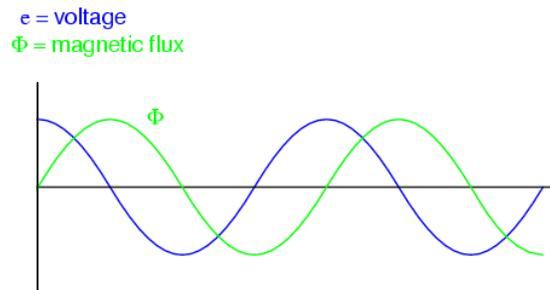
Figure 4: Voltage induced in a coil due to sinusoidally varying flux
