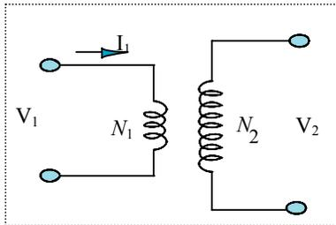
Figure 13(a): Step-up transformer
