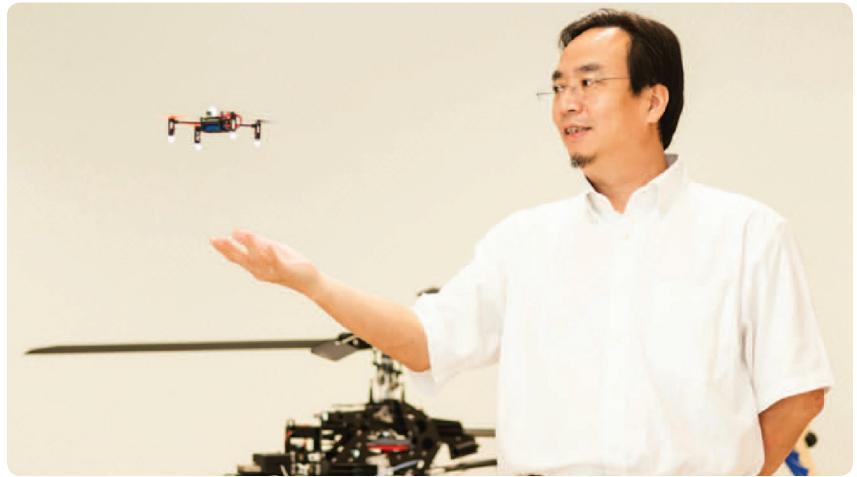
Ben M. Chen and his 40-g fully autonomous microaerial vehicle (photograph courtesy of X. Dong).
